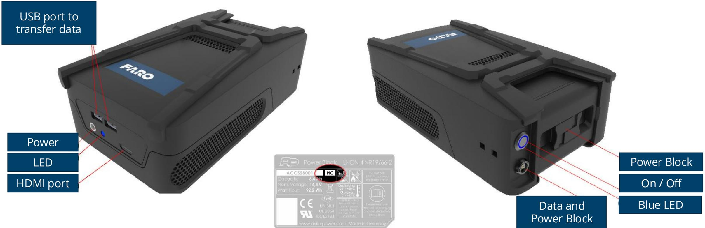
**NOTE:** Older versions of the Power Block are not compatible with the Mobile PC and Freestyle 2. Ensure that your Power Block type label includes the designation HC
