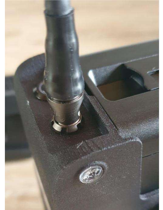
**!** Do not connect or disconnect the FS while Mobile PC is on. Always switch off the Mobile PC before connecting or disconnecting
